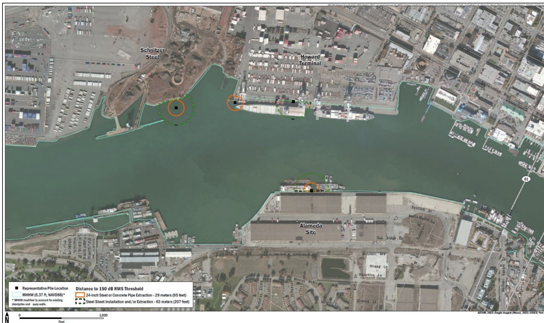
Figure 40: Estimated Distance to In-Water Sound Pressure Criteria for Fish for Vibratory Driving
